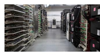
NOVONIX Ultra-High Precision Coulometry (UHPC) systems offer the most advanced and precise battery testing equipment in the industry. Our systems are fully capable battery cyclers that allow our customers to test electrochemical processes within cells rapidly and in various formfactors, providing them with robust data that can improve decision making about their development programs.
